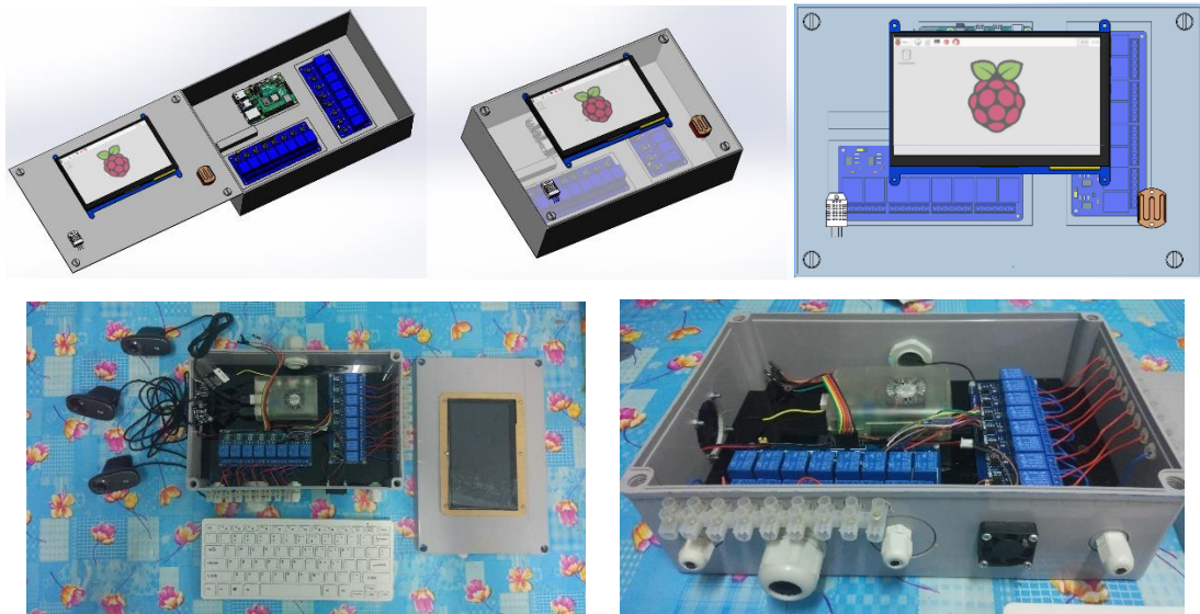
Figure 3.41. Control Panel Box Design
