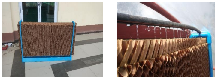
Figure 3.15. Cooling Pad Design
