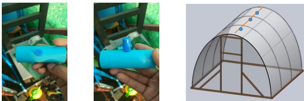
Figure 3.16. Fog Nozzle Sprinklers and Its Placement
