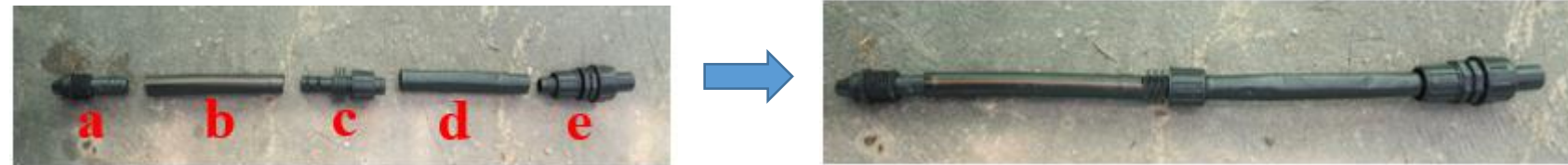
(a) Offtake with rubber, (b) LDPE pipe, (c) Male thread adaptor, (d) 12 mil dripline, (e) Flushing valve
